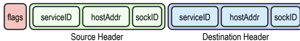
Figure 1: The SCAFFOLD packet header, with a decoupling between who (the serviceID ), where (the hostAddr ), and which connection (the socketID ). Other fields like packet length, version number, and checksum are omitted for simplicity.
