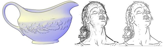
Figure 10: Rendering with suggestive contours. For relatively smooth objects (left), the object-space algorithm produces good results. For noisier input data, we begin with the results of the image-space algorithm (middle), then remove small connected components (right).
