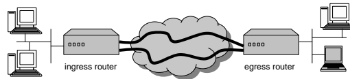
Figure 1: End-routers of a network path, hosts served by those routers, and IP paths connecting the routers.
