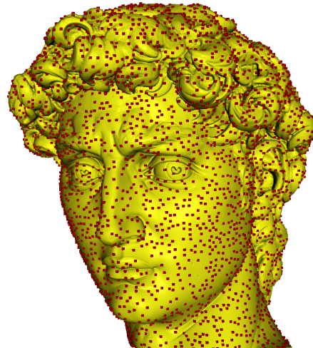
Figure 2. The head of Michelangelo's David, aligned using our non-rigid, global alignment method. The green points are the global feature points used.
