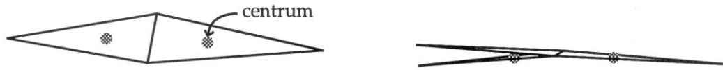
Figure 5.7: In 3-d, if a neighboring hyperplane intersects a centrum for a facet, the facet's vertices are at most 3\rho from the hyperplane.
