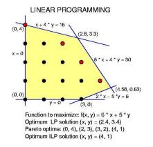
Figure 1: A system of linear inequalities and its feasible region
